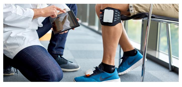
Our **Fesia Walk** patented product for drop foot patients has a **16 pad electrode** attached to the garment. The garment embraces the shank just below the knee. The system also includes an Inertial Measurement Unit (IMU) sensor located and tied to the users shoe laces that **continuously monitors** the gait movement of the leg and **determines the right point of time when the stimulation for dorsiflexion should be applied.**
