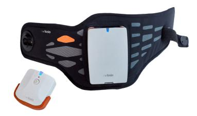
The stimulator communicates with a PC, tablet or smartphone using serial communication over **Bluetooth**, a wireless interface. It can modulate the electrical impulse in **frequency**, **amplitude**, **pulse width and pulse compensation**. Each one of the pads is **fully controllable** and thus **asynchronous activation of motorneurons** is possible, which is important for **fatigue reduction**.
