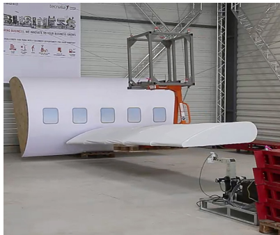
Automated assembly of large parts controlling the rotations
