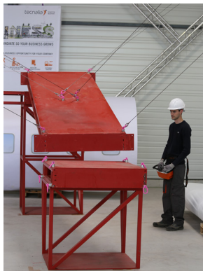
Manually controlled cable driven robot by one person, performing assembly operations
