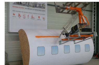
Painting on a curved surface with a robot arm mounted on the cable-driven robot's mobile platform
