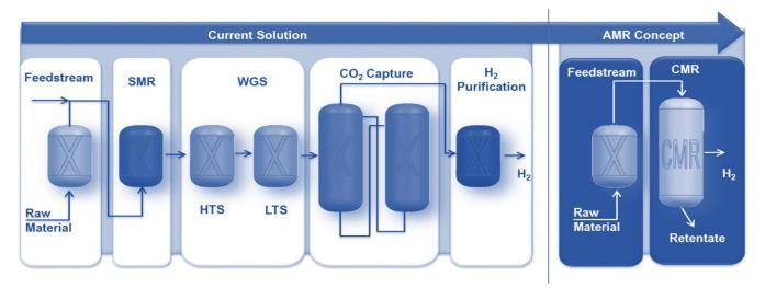
This Advanced Membrane Reactor has been developed for pure hydrogen production at small to medium scale. **AMR integrates in catalytic membrane reactors, reaction and separation in a single stage,** separating the H<sub>2</sub> while it is produced thus shifting the equilibrium towards the products allowing the reduction of process temperature down to less than 600°C.
