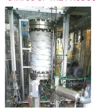
AMR will reach TRL 6 before the end of 2018, with a reactor of 2  $m_{H2}^3$  / h of installed generation capacity.
