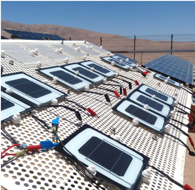
ARGICOAT on silicon solar cell prototype exposed for energy monitorization
