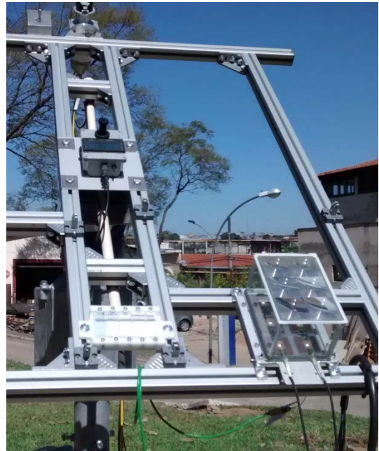
ARGICOAT on multi-junction cell CPV-prototype
