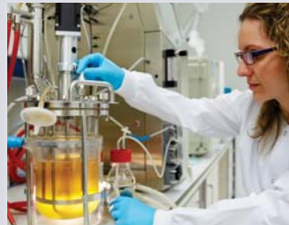
Reactor (10L) for synthesis of ionic liquids.
