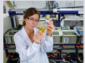
Pilot (15 tanks of 20L) for electrodeposition of metals
