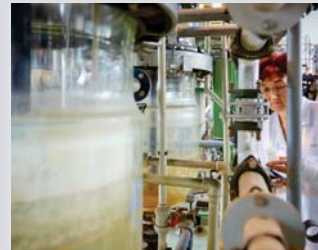
Reactor (100L) for extraction of metals from wastes using ionic liquids.
